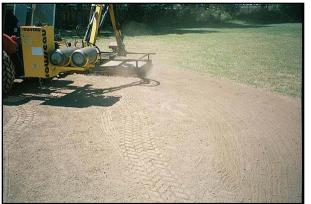
**Above**: **Sunburst's** original boom mounted unit (4'x5') attached to a 55 HP tractor; beginning 3rd treatment to continue removal of well-established grass clumps.
