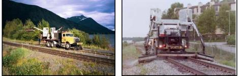
**Above:** hi-rail truck outfitted with two four foot, boom-mounted thermal units and I eight foot wide center, frame-mounted thermal unit. **Left**: preparing for work. **Right**: at work: note spray from perimeter watering system. Mounting of units to booms and set-up of supporting systems provided to the railroad by a fabricator in Anchorage, Alaska. Initial training of work crews and consulting to railroad staff with respect to effective use of equipment provided by **Sunburst**.
